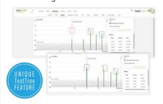
On Transmission site for quick identification of which TX is out of sync: • RF signal Time & Frequency synchronization Before modulation: Distribution Network Delay for MND tuning In SFN overlapping areas for actual Field Reception Quality by Channel Impulse Response monitoring with TestTree's Unique Echo Pattern monitoring mode for a more reliable Echo identification
