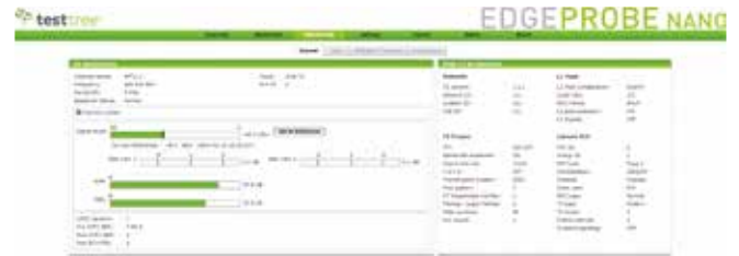
DVB-T2 RF Channel monitoring view
